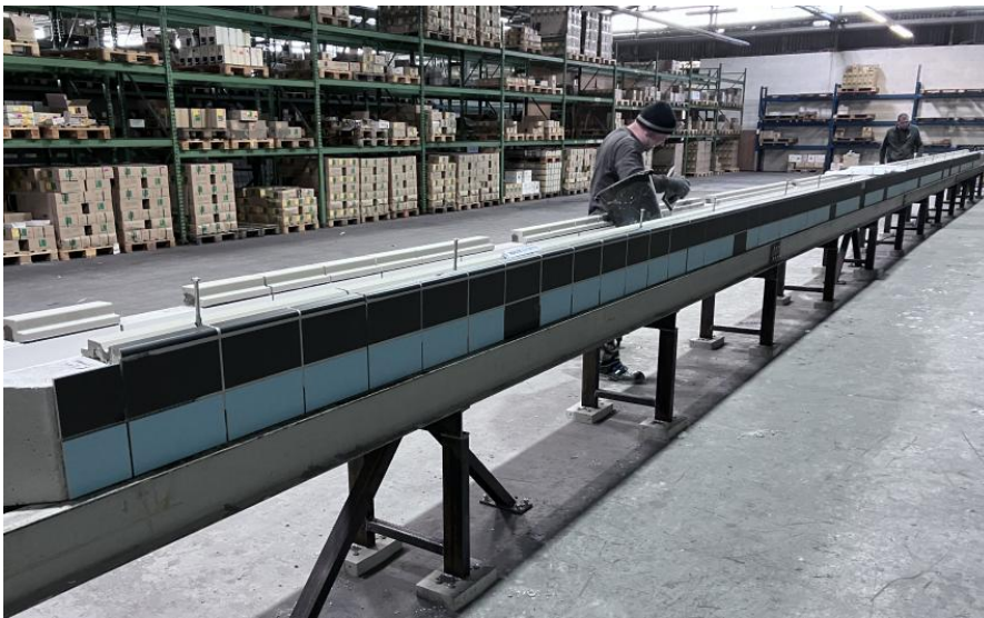
Tiling work on prefabricated components ©agrob-buchtal.de
